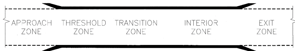
Figure 1. Layout of Tunnel Zones
